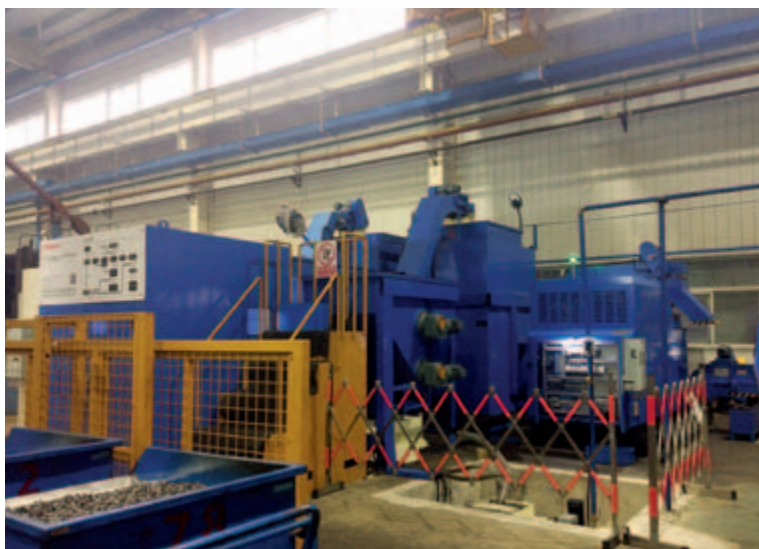
Iron scrap handling and centralized oil supply system
